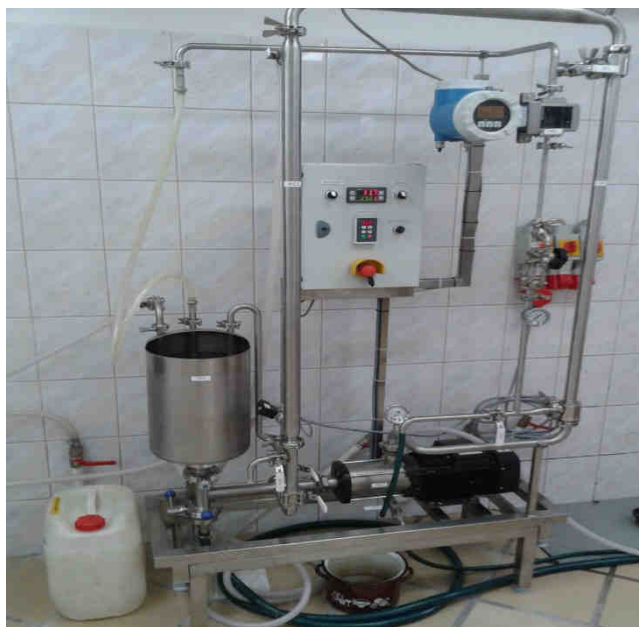
Fig. 1. Membrane installation used in experiments (author: Konrad Cwirko)
