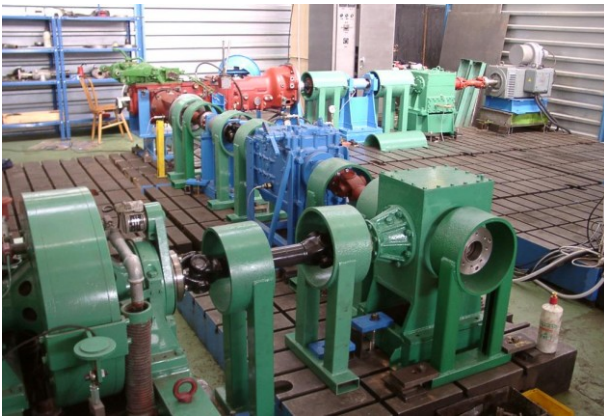
Figure 11. General view of the test rig to measure the efficiency of a power transmission system
