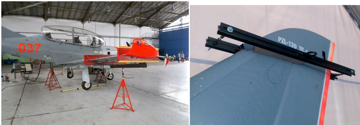
Fig. 5 Wing sensors calibration. Clamps used for wing and fin loading
