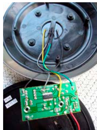
Figure 2. Electronics for lamp (top) with light sensor (bottom)
