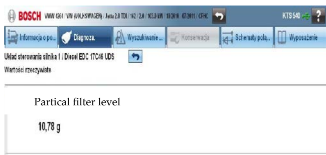
Figure 4. Measurement of the degree of particulate filter contamination
