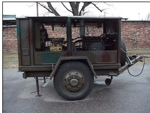
Fig. 4. The supply system for underwater works security base "ORTOLAN" with diving air compressors EK 2-150 manufactured by the USSR.
