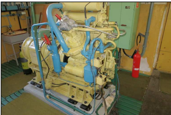
Fig. 3. Diving air compressor EK 7.5-3 manufactured by the USSR.
