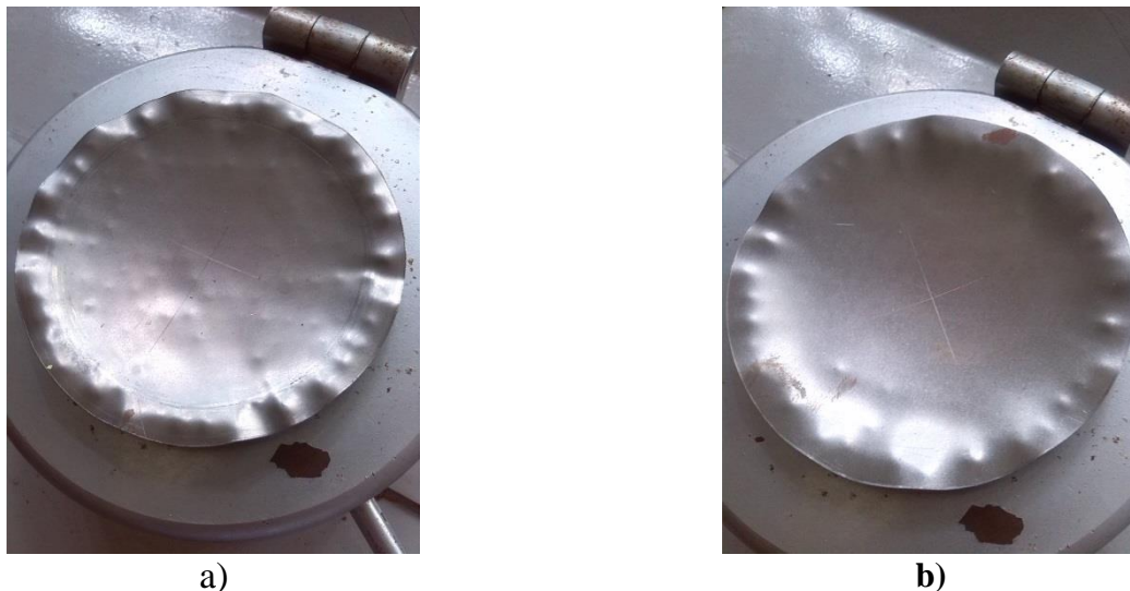
Fig. 9. Hydro-multipoint forming part deformed: a) - without interpolator, b) - with interpolator
