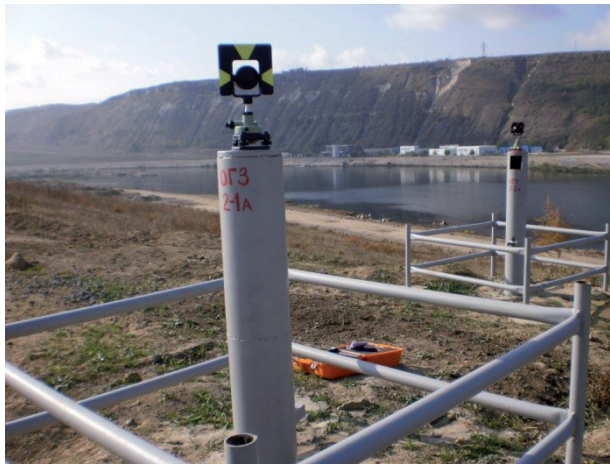
Fig. 1. Points of the control geodetic network on Dniester HPPS
