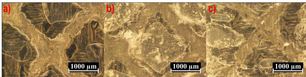
Fig. 3. Microscopic images of heat-sealed films a) PE20, b) PE/Be20, c) PE/B20
