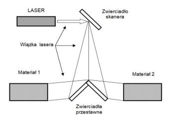
Fig. 7. The Scheme of laser butt welding of polymers [2]
