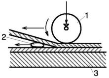
Fig. 1. Scheme of foil welding with a hot wedge, 1 - pressure roller, 2 - heating wedge (pressure), 3 - washer
