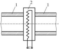
Fig. 2. Scheme of welding by means of a heated plate [2]: 1 - joined elements (pipes), 2 - heated plate (flat)
