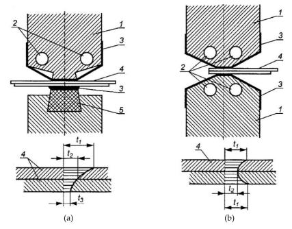
**Fig. 4**. Scheme of polymers foil welding and temperature distribution in welded materials [2], a) heating by means single electrode, b) heating by two electrodes, 1 - electrode, 2 – heating elements, 3 – PTFE pad, 4 – foil, 5 – rubber pad;  $t_1$  –electrode temperature,  $t_2$  – temperature of welding,  $t_3$  – lowest temperature of welded foil.
