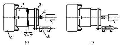
**Fig. 3.** Friction rotary welding of polymers [2]: a) before the welding process, b) welded elements; l –rotating welded element, 2 - immobile welded element, 3 –rotating center, 4 - switch, 5 – spindle centering handle
