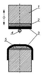
**Fig. 5.** Scheme of impulse welding with cutting off [2]: 1 – pressure bar, 2 – porous rubber spacer, 3 – PTFE spacer, 4 – wire, 5 – impulse tape
