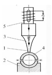
**Fig. 6.** Scheme ultrasonic direct welding [2], 1 – sonotrode, 2 – anvil, 3 – waveguide, 4 – welded elements, 5 – ultrasonic transformer
