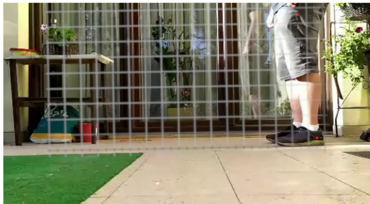
Figure 1. Frame 1 from the left profile perspective (XY coordinate system). Markings: red dots - measuring characteristic points, the size of one grid in the auxiliary grid is 1x1 [dm]. Source: Own measurements made with the Xiaomi Redmi Note 7 phone [12, 26].
