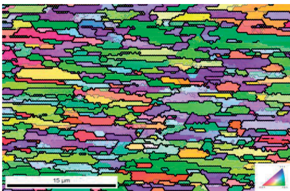
Fig. 28. Map of grains and map of crystallographic orientation distribution in Cu-Ag-Mm alloy
