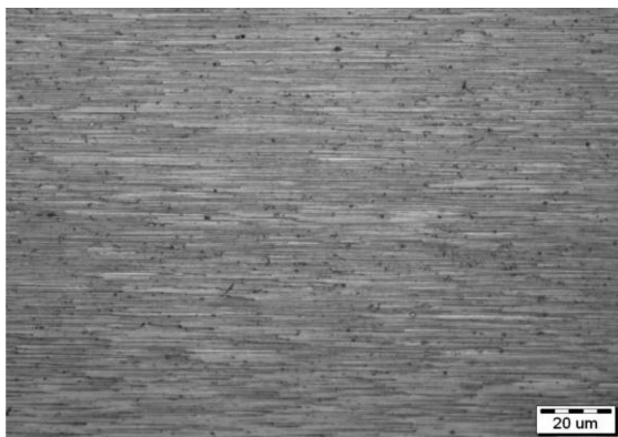
Fig. 19. Microstructure of Cu-Ag-Mm wire of diameter 0,5 mm after heat treatment in 200°C/7h, longitudinal section
