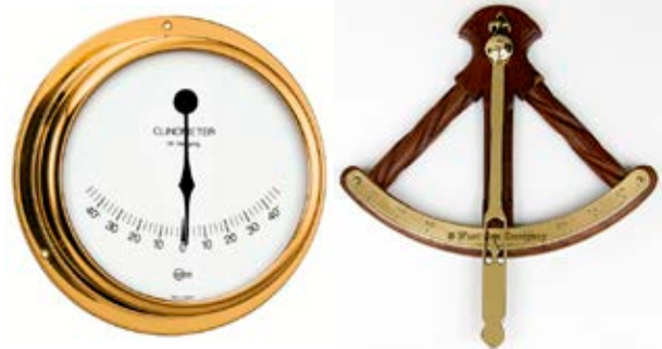
Figure 2. Selected clinometers used onboard of LNG carrier (Sea shop, 2016; West Sea Company, 2016)
