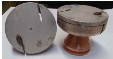
Fig. 6. Contacts after some 15 kA short circuit current interruptions
