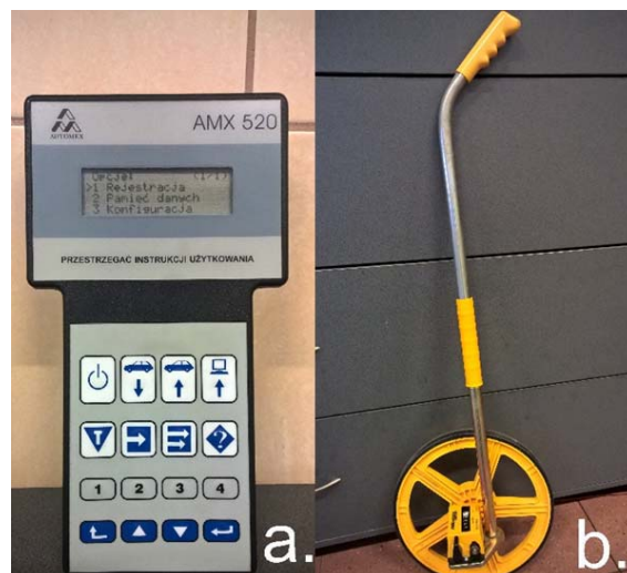
Fig. 4. Measuring instruments a) AMX 520 decelometer and b) Trumeter 5500 road measuring wheel
