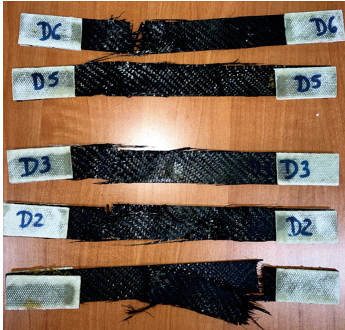
Figure 5. D-series composite specimen after tensile strength tests [op. cit.]
