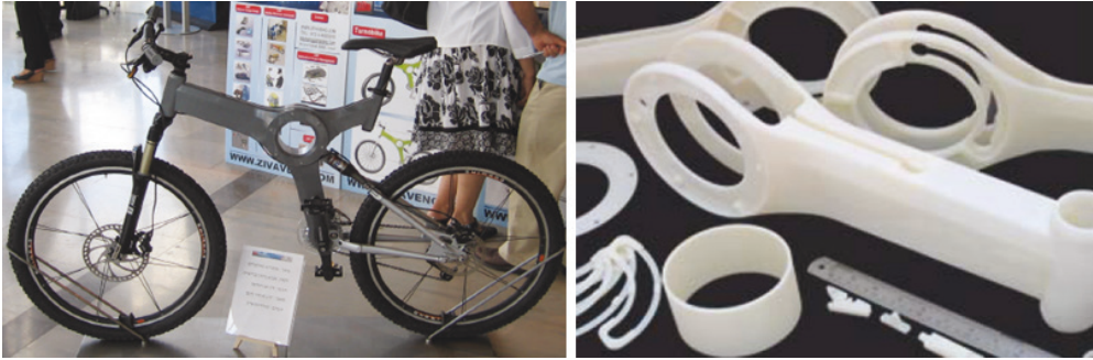
Fig. 2. 3D printed bicycle with Solido LOM 3D printer (source: www.drukarki-3d.info )
