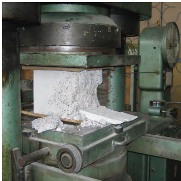
Fig. 3. Compressive strength test of the product modified with basalt aggregate
