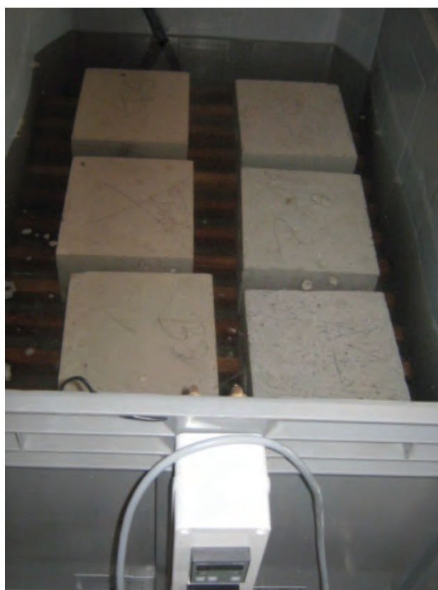
Fig. 4. Absorption test of the traditional and modified products
