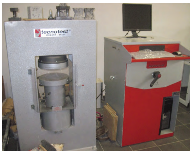
Fig. 2. Hydraulic Press – compressive strength test, Kielce University of Technology
