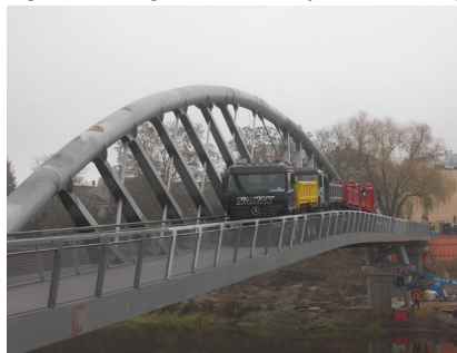
Fig. 10. Static proof load test of the structure (scheme U2).
