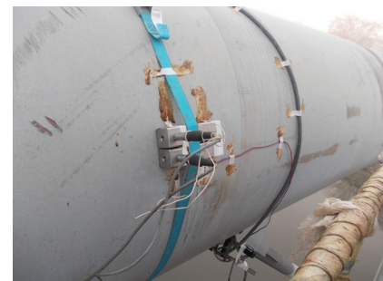
Fig. 5. Accelerometer B12/200 – measurement of vertical and horizontal accelerations of the deck (on the left) and measurement of horizontal accelerations of the arch (on the right).
