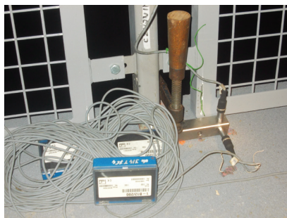
Fig. 5. Accelerometer B12/200 – measurement of vertical and horizontal accelerations of the deck (on the left) and measurement of horizontal accelerations of the arch (on the right).
