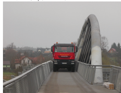
Fig. 9. Inducing of vibrations by half-crouching with frequency f_1 (the arch).
