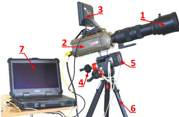
Fig. 5. View of the optical head with the portable PC (7): lens (1); camera (2); display (3); pan and tilt mechanism (4); angle reading system (5); tripod (6)
