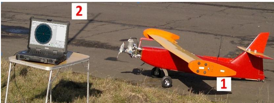
Fig. 1. Main system components: the acoustic locator (1); the ground unit (2)
