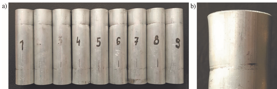
Fig. 14. Deformations on the sleeves: a) in the pressure zones of the chord walls at the location of the larger holes, b) deformation of the head of sleeve no. 7
