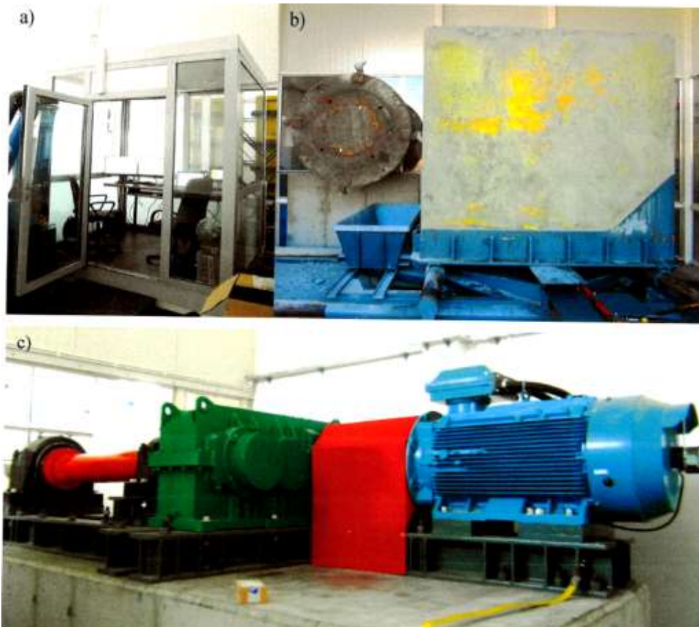
Fig. 12 Laboratory workstation for testing by cutting or rotary drilling with single cutting tools or heads: a) operator's cab, b) concrete sample with an assembly for its mounting and feed as well as a test cutting head; c) head drive
