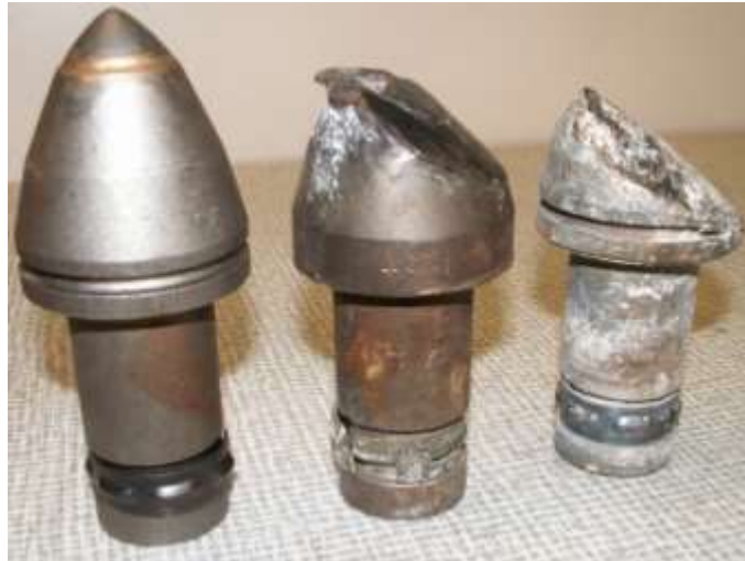
Fig. 8 Improperly worn (asymmetrical) conical picks
