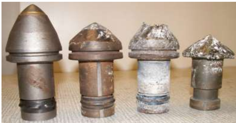
Fig. 6 Properly worn (symmetrical) conical picks
