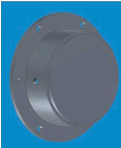
Fig. 12. Cylinder for the injection of the sealing medium
