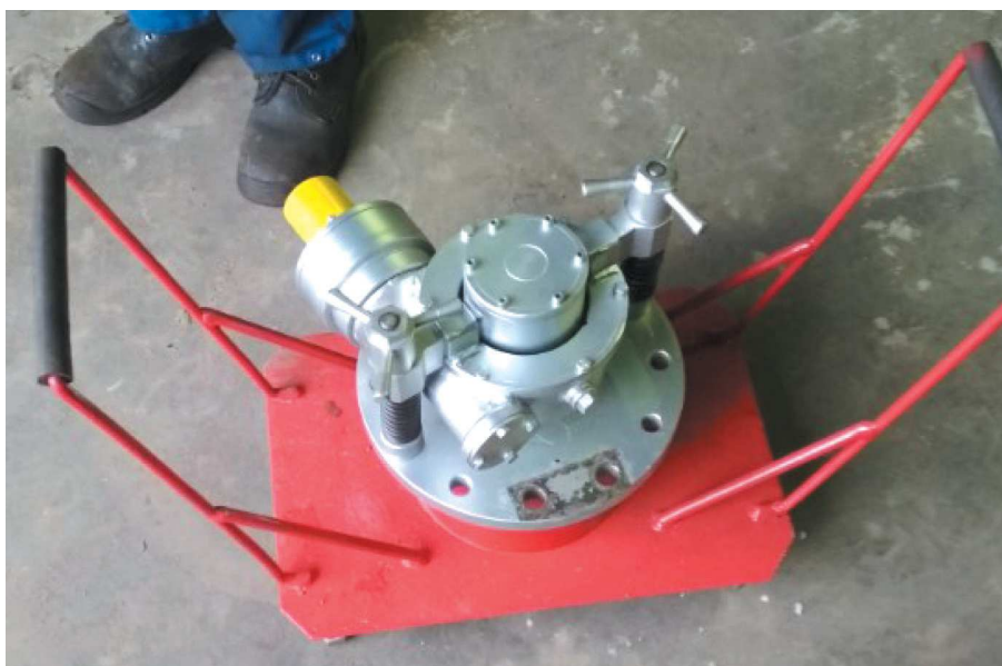
Fig. 13. Basket used for the milling machine transport
