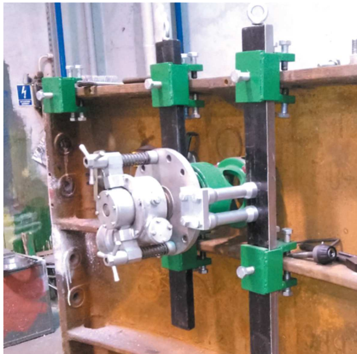
Fig. 4. Milling machine mounted to tubing
