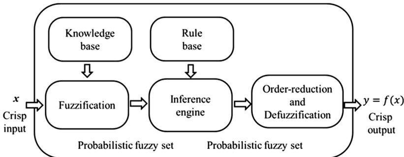
Figure 1: Probabilistic Fuzzy Inference System – structure
