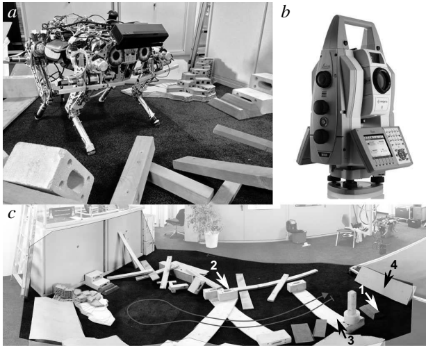
Fig. 16. Experimental setup with the quadrupedal robot StarLETH (a), laser scanner Leica Nova MS50 MultiStation ( leica-geosystems.com ) used for ground truth recording (b), overview of the experimental terrain (c).
