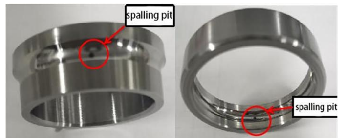
Fig. 10. Simulation topography of bearing fatigue spalling fault.
