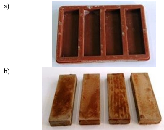
Fig. 3. Wax pattern (a) to make standard reference ceramic samples (b)
