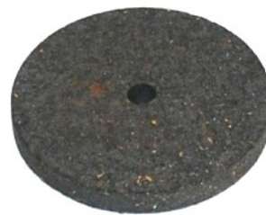
Fig. 5. Counterface disk made of friction material JT6500 (photo by the authors)
