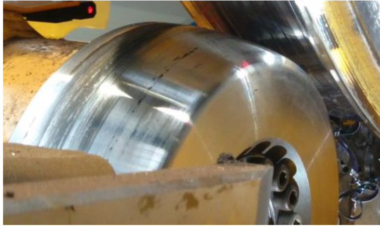
Fig. 9. The drive roller with clear traces of wear (with the consent of PPW KOLTECH)
