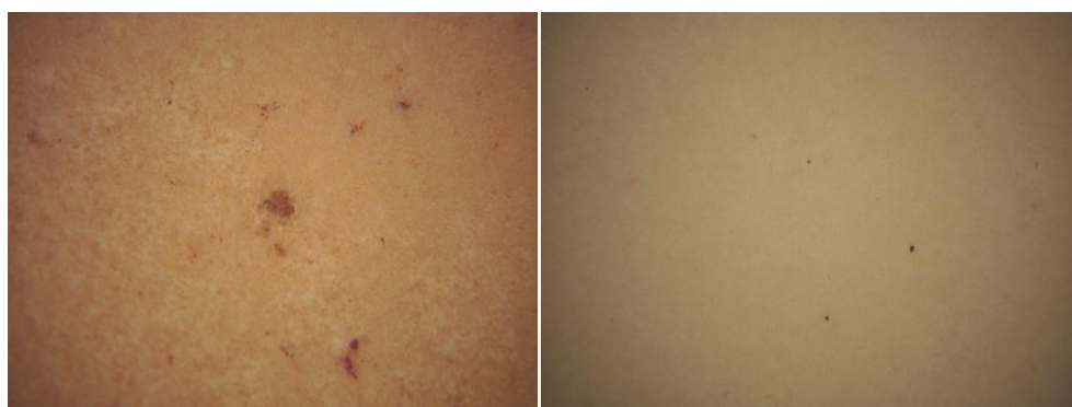
Fig. 14 Merox fuel deposits > 3.0 \mu\text{m} (zoom 11x)
