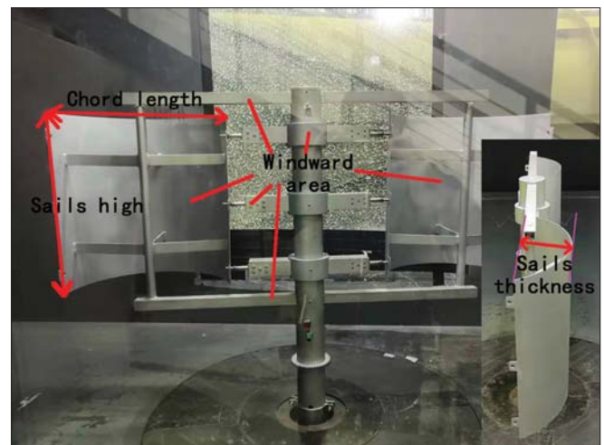
Fig. 3. Basic parameters identification of multi-mode sailing device
