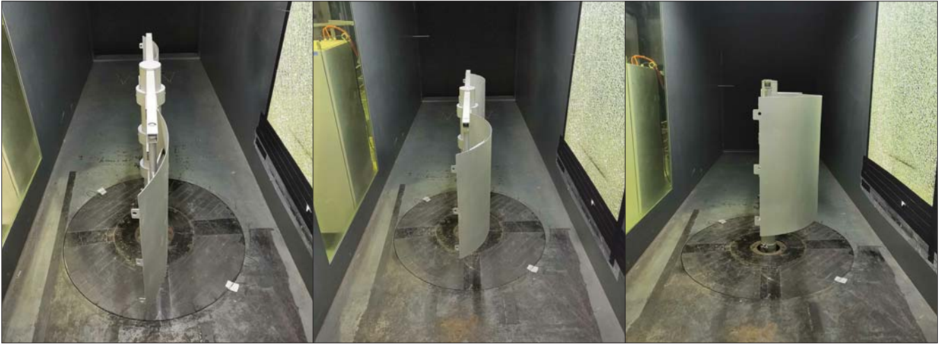
Fig. 2. Installation's diagram of a multi-mode sailing device in the wind tunnel
