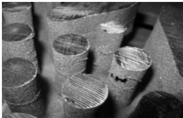
Fig. 6. Burrs on connections on cut casting [4]
