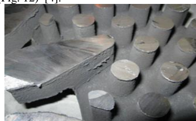
Fig. 12. Places of burrs occurrence by present production [4]
