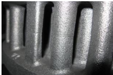
Fig. 5. Connections on castings with the use of additive BR 4048 [4]
