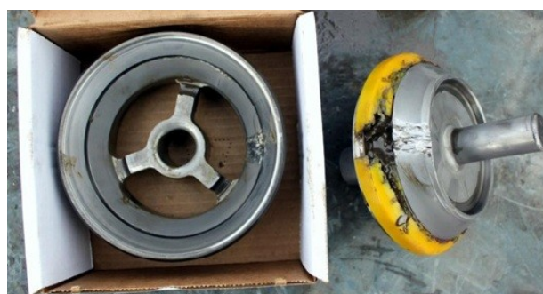
Fig. 8. Damaged seat and head of a mud pump valve [5]
