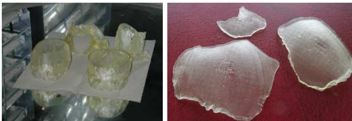
Rys. 8. Modele wykonane metodą SLA [6], [10] Fig. 8. Model made with SLA technology [6], [10]
