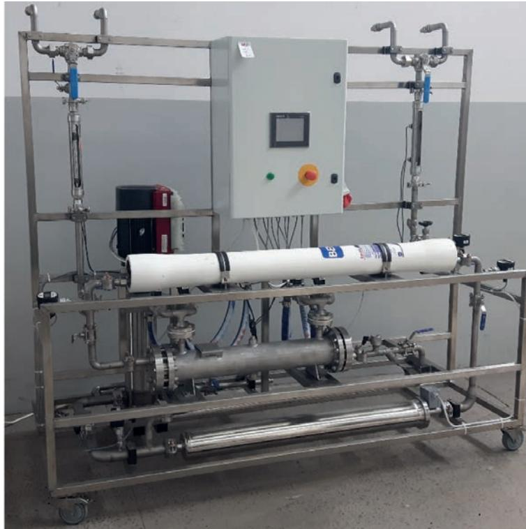
**Fig. 7. Prototype membrane ultrafiltration plant**
