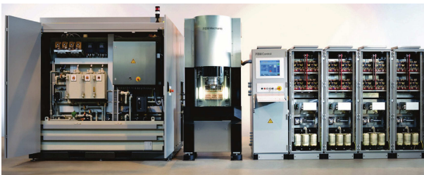
Fig. 4. Modular electrochemical machine-tool offered by PEMTec [16].
