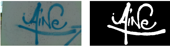
Fig. 2. Image processing: colour frame (left) and corresponding binary mask (right)
