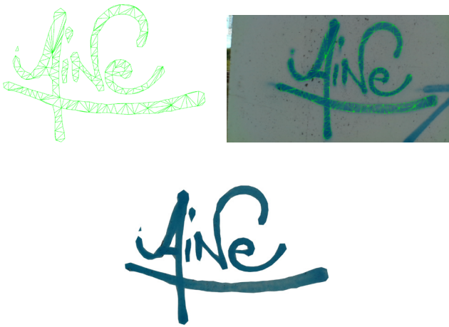
Fig. 5. Decimated mesh (top left), mesh mapped texture (top right), and textured mesh (bottom)
