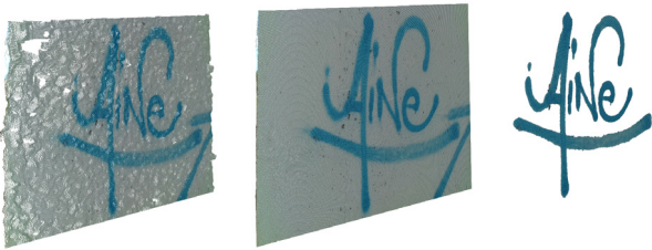
Fig. 3. Point cloud processing: original point cloud (left), point cloud projected on to a plane fitted with RANSAC (middle), and point cloud representing the segmented defect (right)
