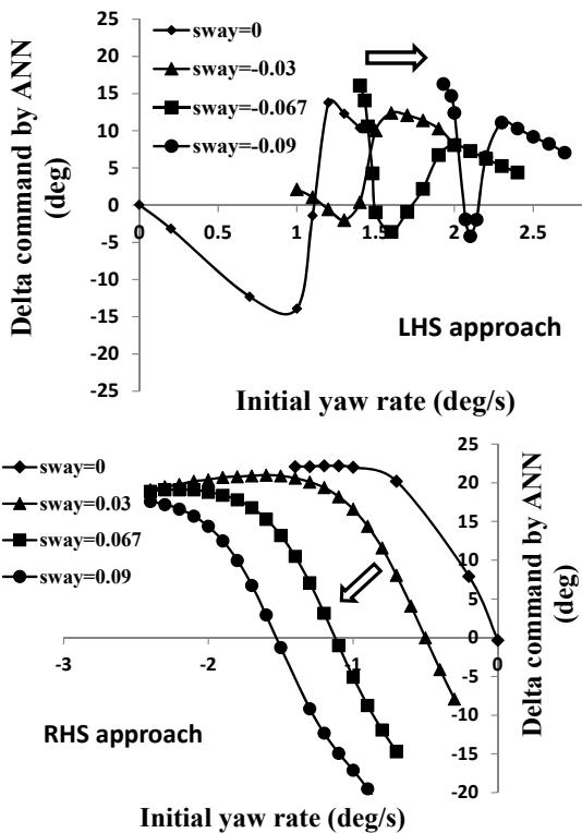
Figure 12. ANN's response for different sway velocity and yaw rate
