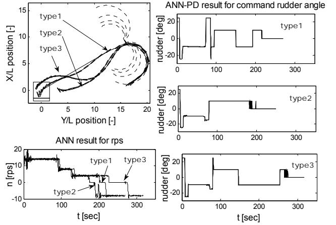
Figure 10. Berthing experiments for RHS approach
