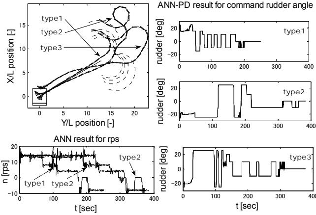
Figure 9. Berthing experiments for LHS approach
