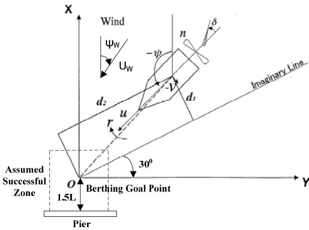
Figure 1. Coordinate system and other assumptions during berthing
