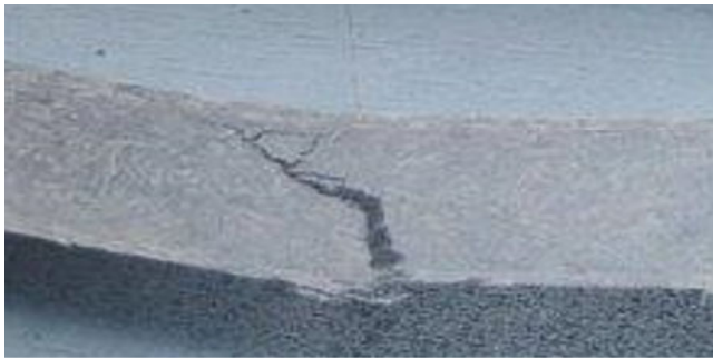
Fig. 8. Example of failure form of a specimen subjected to 3-point bending
