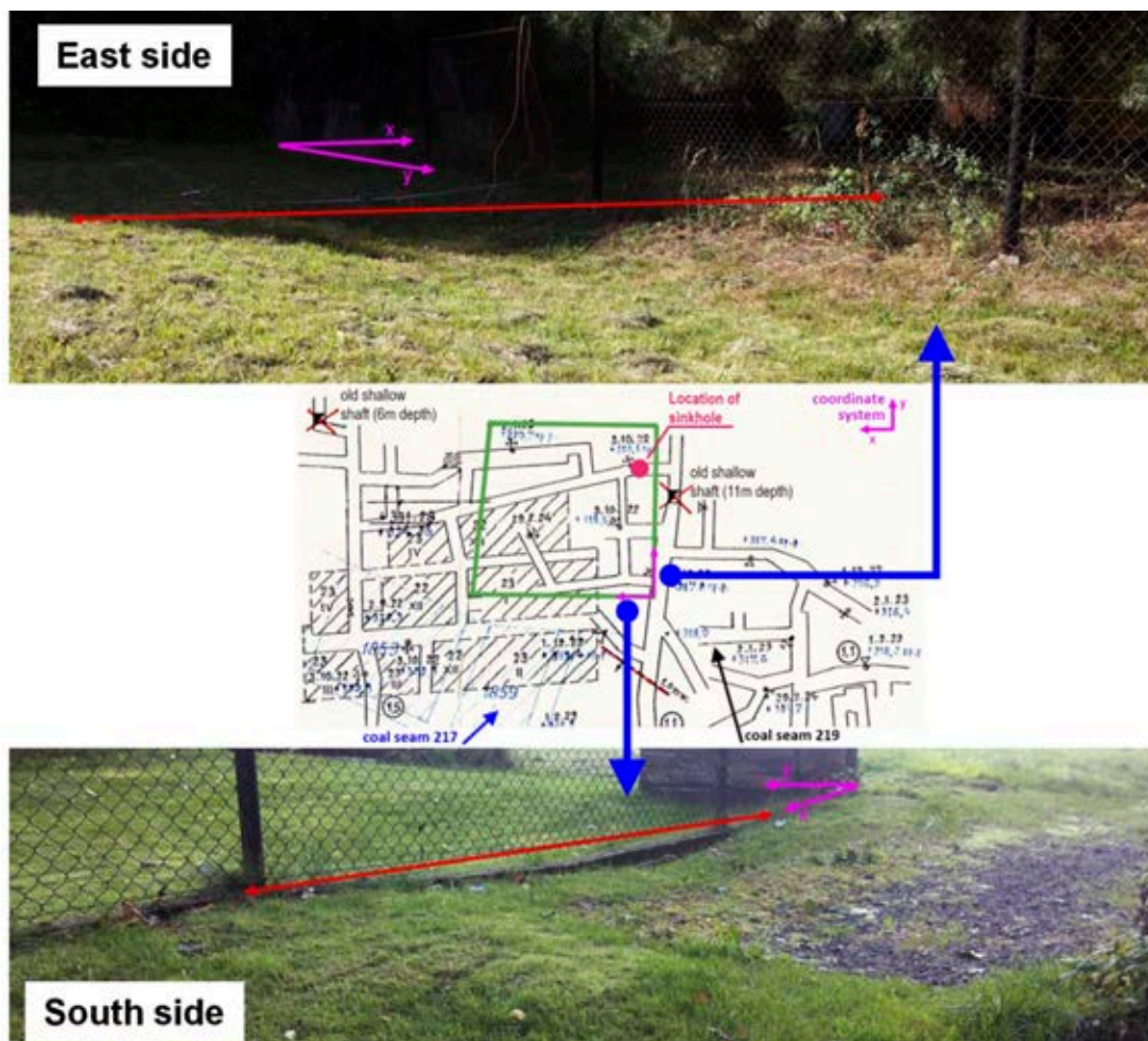
Figure 6. Deformations observed on the surface: micro-subsidence troughs (cover-subsidence sinkholes) near the border of the plot
