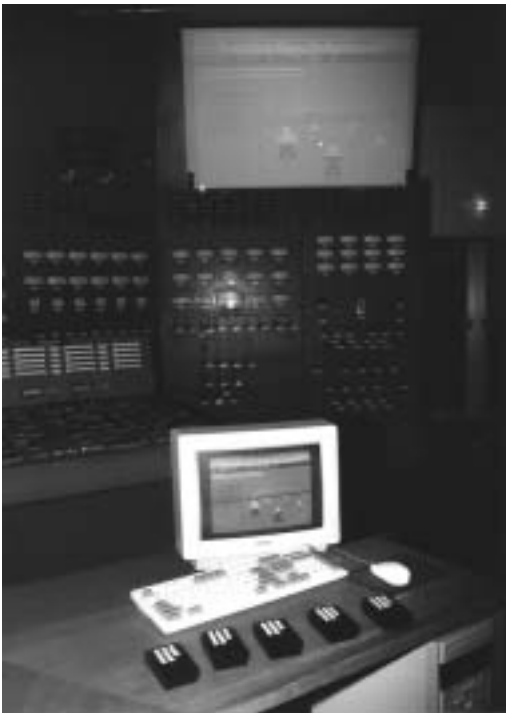
Figure 2. Hardware elements of COSMOS. Both the personal computer display and the large projector screen show the summarised result of the team evaluation in a graphical form.
