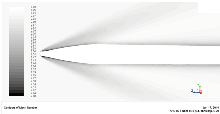
Fig. 4. Flow velocity map depicted in terms of the Mach number [Bednarczyk, 2014]
