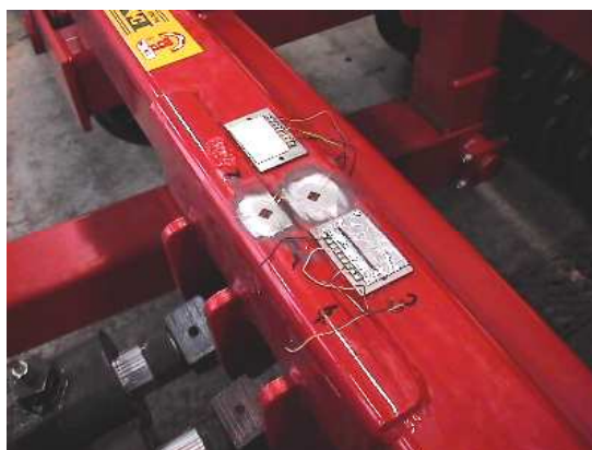
Rys. 5. Tensometry naklejone na belce wózka jezdnego Fig. 5. Strain gauges stick on roller chassis beam
