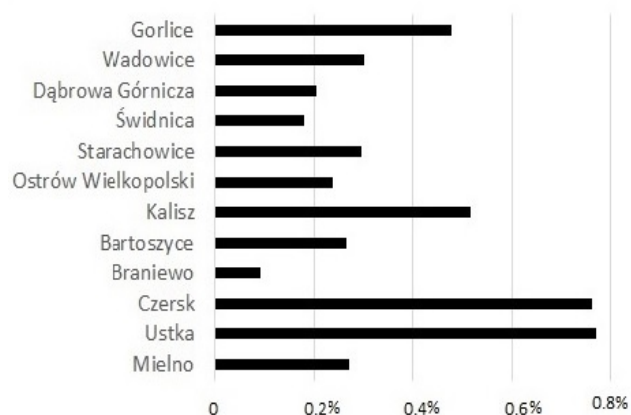
Fig.4. Percentage share of electricity consumption by road lighting installations in total electricity consumption. Source: Own study
