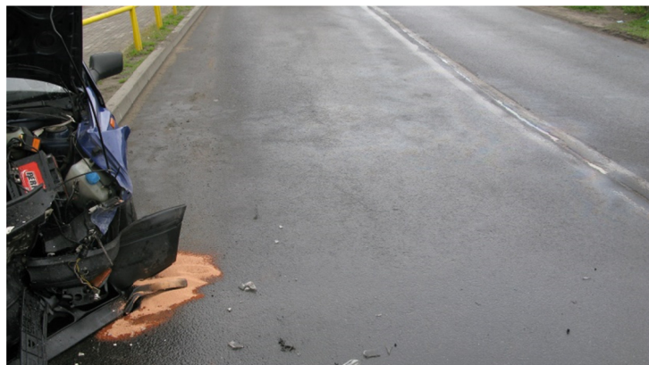
Fig. 2. View of the asphalt roadway wet polluted with diesel
