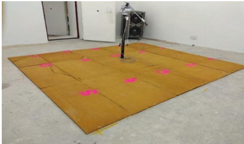
Figure 1. Reverberation chamber B. Sample - Fiberboard 20mm.
