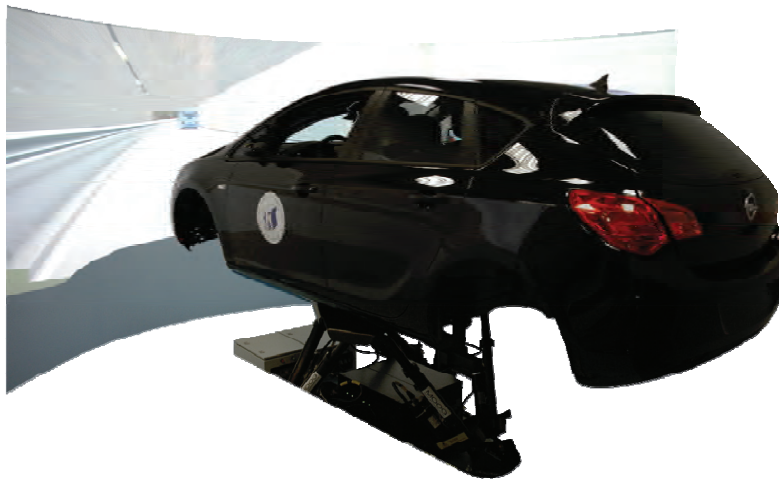
Fig. 2. AutoSim AS 1200-6 advanced high-class car simulator
