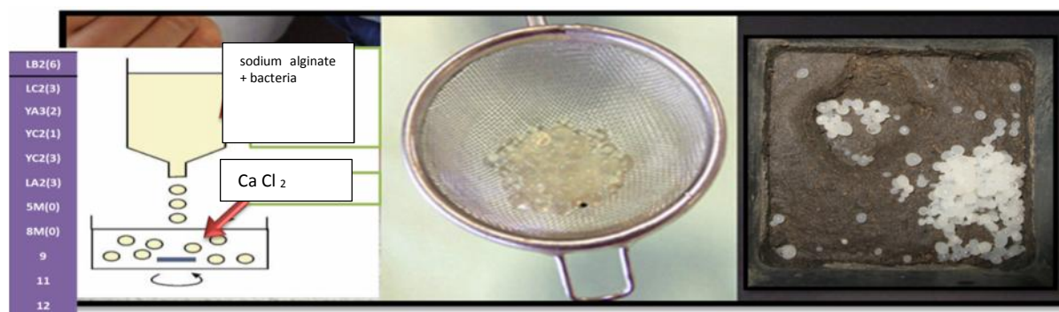
Fig. 1. The production of the biopreparation for plant growth stimulation is based on the technology regarding the immobilisation of micro-organisms on media
