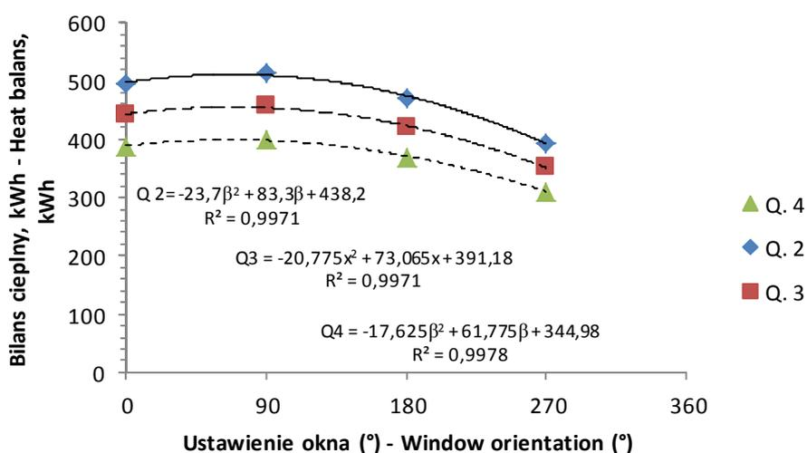
Fig. 1. Summer heat balance  $Q$  of double ( $Q_2$ ), triple ( $Q_3$ ) and quadruple ( $Q_4$ ) glazed windows facing different geographical directions (0 – east, 90 – south, 180 – west, 270 – north)
