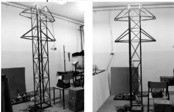
Fig. 2. Laboratory physical model of the transmission tower construction
